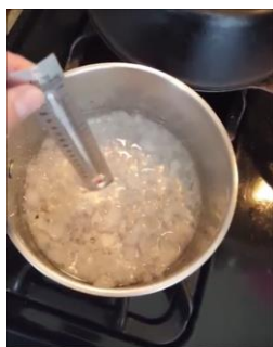
In this phase changes lab scholars record the temperature each minute as they see water go from a solid to a liquid to a gas state.
