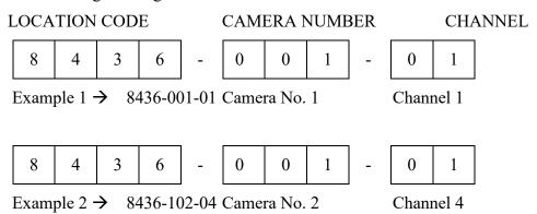
B. Weather proof labels showing the corresponding camera number shall be applied to each camera's housing.
