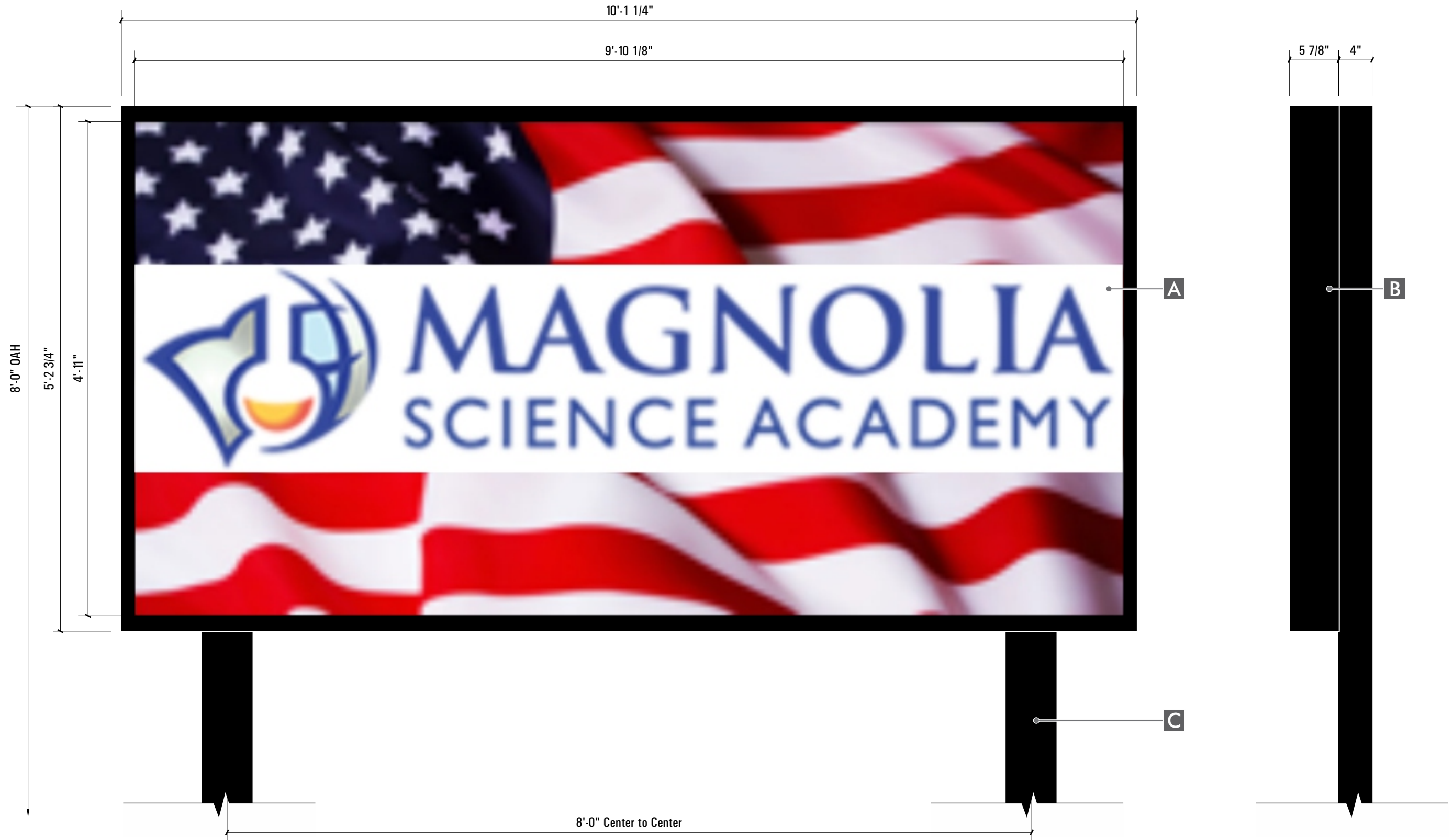
A B TWO (2) POLE MOUNTED S/F SAMSUNG PRISMVIEW XPR-B 12X6 SCALE: 1" = 1'-0"
