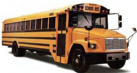
**TYPE C:** A Type C school bus is constructed utilizing a chassis with a hood and front fender assembly. The entrance door is behind the front wheels—also known as a conventional-style school bus. This type also includes the cutaway truck chassis or truck chassis with cab with or without a left side door and with a GVWR greater than 21,500 pounds.
