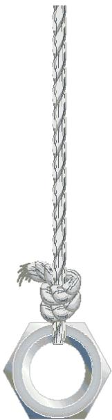
**Note:** It is important to drop the inspection tool over the handrail in such a way as to simulate a child exiting the bus. This is a drop-and-drag test. Do not create a snagging situation by placing the nut in an area that would not be exposed to a drawstring or other articles.
