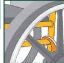
▼ **Do not attach tiedowns to adjustable, moving, or removable parts of the wheelchair such as arm supports, foot supports, and wheels.**
