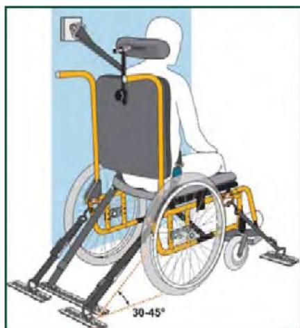
▼ It is important to use a complete WTORS to secure the wheelchair and provide the wheelchair occupant with a properly fitting lap and shoulder belt system.
