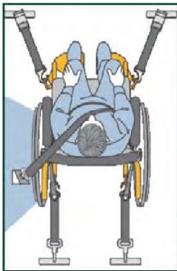
▼ When securing non-WC19 wheelchairs, choose structural securement points as close to the seat surface as possible to provide greater wheelchair stability during travel. It is best if the rear securement points are high enough to result in angles of the rear tiedown straps between 30 and 45 degrees to the horizontal.
