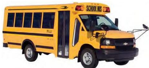
**Type A-1,** with a Gross Vehicle Weight Rating (GVWR) of 14,500 pounds or less; and
