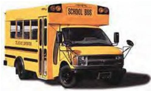
**TYPE A:** A Type A school bus is a conversion bus constructed utilizing a cutaway front section vehicle with a left side driver's door. This definition includes two classifications: Type A-1, with a gross vehicle weight rating (GVWR) of 14,500 pounds or less; and a Type A-2, with a GVWR greater than 14,500 pounds and less than or equal to 21,500 pounds.
