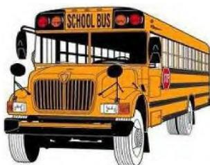
**Type C:** A Type "C" school bus is constructed utilizing a chassis with a hood and front fender assembly. The entrance door is behind the front wheels; also known as a conventional school bus. This type also includes cutaway truck chassis or truck chassis with cab with or without a left side door and a GVWR greater than 21,500 pounds.
