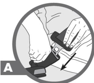
**A** BUCKLE the latch plate into the matching buckle after lifting the lap belt webbing from the seat and lengthening the lap belt strap. To lengthen the strap, tilt the latch plate and pull it along the strap. LISTEN for the CLICK sound when the latch plate is fastened!
