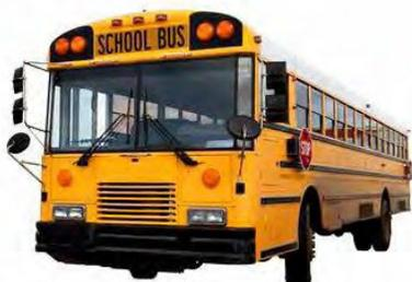
**Type D:** A Type D school bus is constructed utilizing a stripped chassis. The entrance door is ahead of the front wheels—also known as a rear-engine or front-engine transit-style bus.
