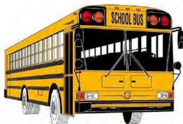
**Type D:** A Type "D" school bus is constructed utilizing a stripped chassis. The entrance door is ahead of the front wheels; also known as rear or front engine transit style school buses.
