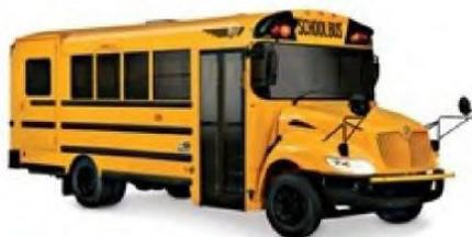
**Type B:** A Type "B" school bus is constructed utilizing a stripped chassis. The entrance door is behind the front wheels. This definition includes two classifications: Type B-1, with a GVWR of 10,000 pounds or less; and Type B-2, with a GVWR greater than 10,000 pounds.
